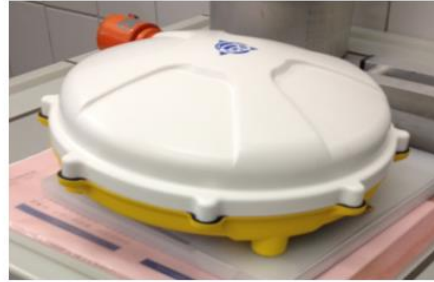
Ryc. 3.48. Odbiornik Trimble SPS 855 oraz antena ZEPHYR Model 2 Rugged, (DGPS specification, 2012)
